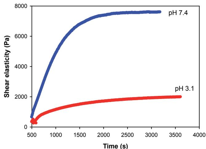
Fig. 3 Gelation kinetics of agar at two different pH values (pH 7.4 and 3.1) at 25 °C by ElastoSens™ X3.
