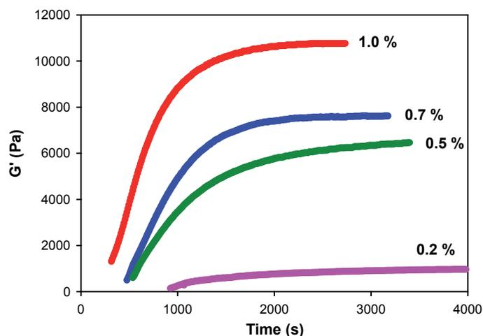
Fig. 2 Gelation kinetics of agar at various concentrations measured at 25 °C by ElastoSens™ X3 (pH 7.4).
