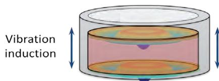
Fig. 1 Principle of ElastoSens™ X3: Non-contact and non-destructive measurement of few micrometers amplitude vibrations.
